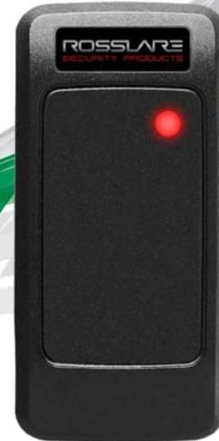
Rosslare's AY-K20B is a powerful RFID proximity card reader of 125-kHz cards and tags, featuring multi-format output and an excellent read range. The reader supports both standard EM and Rosslare format cards, and is highly flexible with behavior control options. With a sleek design and a tough UV-resistant and water-resistant casing, the AY-K20B is equally suited to indoor and outdoor use.
